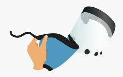
2. Attach the folded neck guard to the central Velcro dot and then secure one half of the neck guard to the visor.
