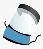
3. Attach the other half, ensuring a secure attachment with no gaps and checking that the neck guard is central to the visor.
