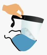
4. Then attach the other half. Ensure a secure attachment with no gaps and that the neck guard is central to the visor.
