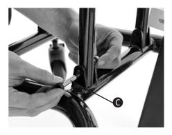
Add the bolts and tighten **G**. Repeat this on the other side. Then lift up the manual actuator to the free lugs on the cross bar and line up the holes, then add bolts and tighten **D**.
