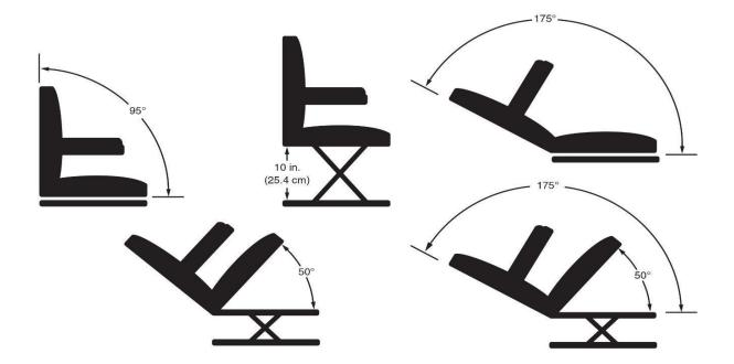
There is a power inhibit on your TRU-Balance<sup>®</sup> 3 Power Positioning System which will not allow you to drive your power chair while in the tilt position. A full inhibit will activate at 20°-50°. See below.
