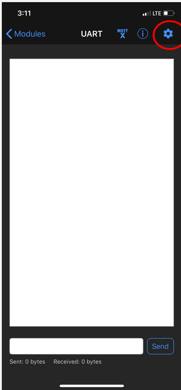
Figure 13 - Once in the UART module, press the setting button in the top right corner.
