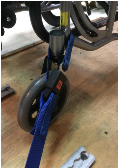
Fitting the Front Restraint
