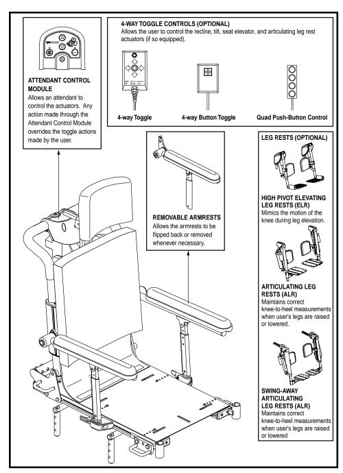
Figure 1. Components of the Synergy TRU-Balance Power Recline
