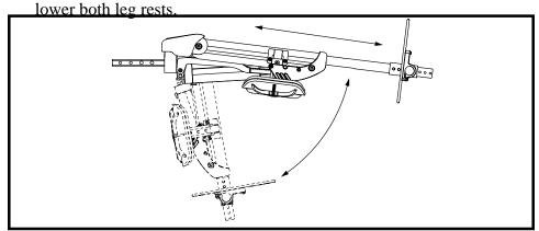
Figure 11. The Power Articulating Leg Rests Option
