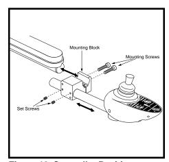
Figure 13. Controller Position - Mounting Block
