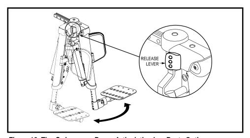
Figure 12. The Swing-away Power Articulating Leg Rests Option
