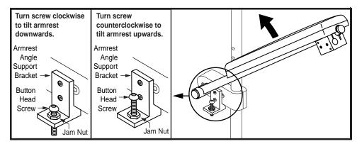
Figure 10. Flip-Up Armrest Angle Adjustment
