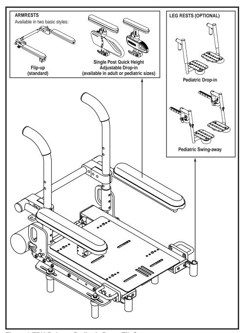
Figure 1.TRU-Balance Pediatric Power Tilt Components
