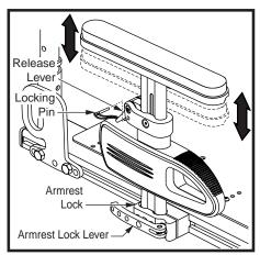
Figure 15. Pediatric Single Post Quick Height Adjustable Armrest Top Height Adjustment
