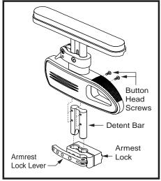
Figure 16. Pediatric Single Post Quick Height Adjustable Armrest Bottom Height Adjustment
