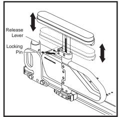
Figure 13. Single Post Quick Height Adjustable Armrest Top Height Adjustment
