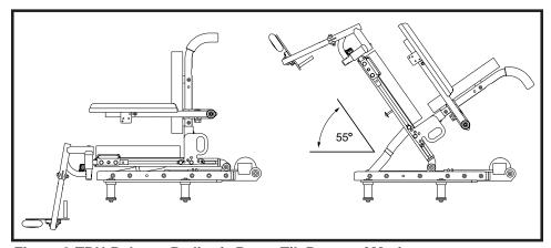
Figure 2.TRU-Balance Pediatric Power Tilt Range of Motion
