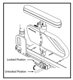
Figure 12. Single Post Quick Height Adjustable Armrest Removal/Installation
