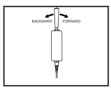
Figure 6. 2-way Toggle Operation
