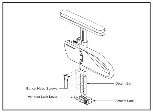
Figure 14. Single Post Quick Height Adjustable Armrest Bottom Height Adjustment
