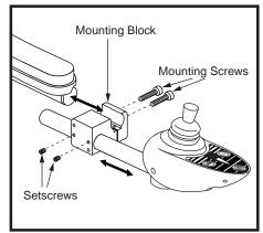
Figure 17. Controller Position - Mounting Block
