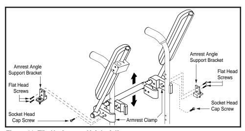
Figure 11. Flip-Up Armrest Height Adjustment
