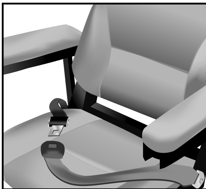
Figure 18. Positioning Belt Adjustment
