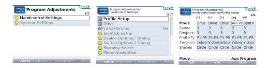
The Click To Phone screen will need to be enabled. Enable this by pressing the green menu key on the joystick to gain access to the menu options (if a light joystick is used then enter the main menu through the Aux screen). Highlight the hand control settings and make a right command of the joystick.
