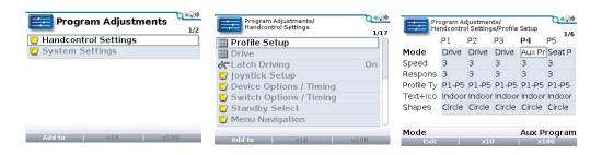
The VoiceOver screen will need to be enabled. Enable this by pressing the green menu key on the joystick to gain access to the menu options (if a light joystick is used then enter the main menu through the Aux screen). Highlight the hand control settings and make a right command of the joystick.
