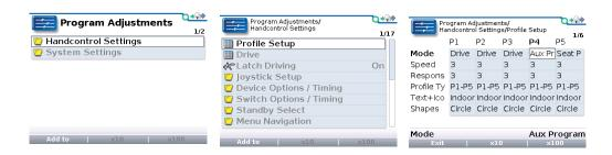
The mouse screen will need to be enabled. Enable this by pressing the green menu key on the joystick to gain access to the menu options (if a light joystick is used then enter the main menu through the Aux screen). Highlight the hand control settings and make a right command of the joystick.
