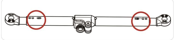
2.3. Select the locations of spring pins according to the desired seat width.
