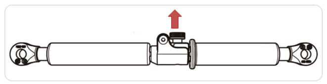
3.2. If the backrest tube is not fordable, the knob nut shall be located on the bottom side.
