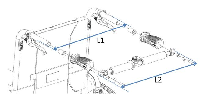
2.1. Push both lateral support bar Foam inwards until all four spring pins can be seen.
