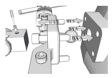
5. Tighten all screws evenly with a 5/32 T-Handle in a clockwise direction.
