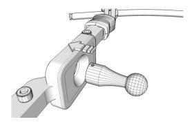
3. Slide 17mm steel ball with swing away hardware back into ball receiver. Retighten tapered set screw with 5/32 T-Handle in a clockwise direction.
