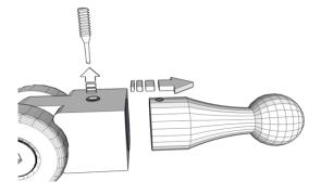
2. Slide backside of ball through SUS center swing away mounting bracket.
