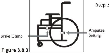
Step 3: Reposition wheel mounting bracket as required. Replace bolts, washers and nuts and tighten. Replace quick-release wheels, loosen brake clamps with a 5mm allen key and slide along frame to suit new wheel position.
