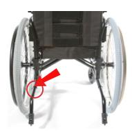
To fit: Depress rear location button on the antitip bar and slide into rear of frame tube. The front button MUST engage through the hole in the frame. Check antitip is secure by attempting to push backward and forward. Follow these instructions to fit the atnitip bar on the other side of the wheelchair.
