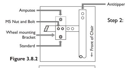
Step 2: Remove the two M6 nuts and bolts with a 5mm allen key and 10mm spanner (as supplied in Karma tool kit).
