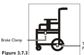
Step 3: Use the larger bottom hole on the block (see fig 3.3.3) to mount the transit wheel. The block should be pointing towards the ground with the flat side of the block facing outwards away from the frame.
