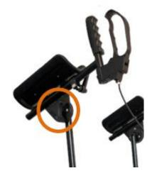
Loosen the star screw on the side until you can move the forearm supports outwards out of the lock. Now you can rotate the forearm supports in the desired angle and push back into the lock. Tighten the star screw again.
