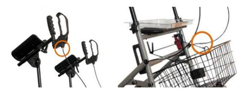
The brake is correctly adjusted when the brake lever as well as the brake wires is free of play and the wheels can be rotated without grinding noises when the brake is released.
