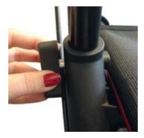
Insert push handles at least to the first cross hole into the frame tubing. Insert the fixing screw from the inside and tighten using the washer and star screw. To change the height adjustment of the push handles, loosen the fixing screw by turning the star screw counter-clockwise. Then lock the handle at the desired height, as described above.
