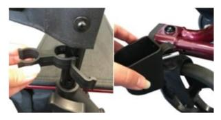
Put the upper cane holder with the pins into the 2 holes at the push handle pipes below the backrest and close the clip. The lower cane holder part must be fixed with the pin in the fixation whole. Make sure correct assembly. The cane holder can be mounted left or right.
