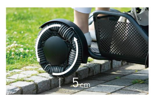
Effortlessly climb over obstacles up to  $5\ \mathrm{cm}$  in height with two powerful motors and large front omni-wheels.
