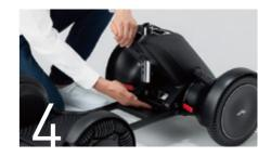
Pull the lever on the side of the battery toward you to separate the parts.
