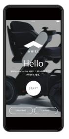
Check your total mileage, distance traveled, battery level, full charge cycles and more with the WHILL app\*. You can also lock and unlock the unit.
