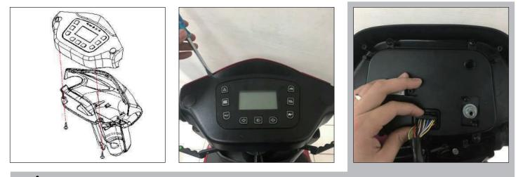
\* If you have problems with the control panel, please reconnect the main cable connector first. If the situation does not change, please replace with a new product immediately.
