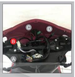
\* Please refer to the previous page for upper control wiring maintenance, and re-connect the connector B of the VR initiator controller. If this has no effect, please replace with a new part.
