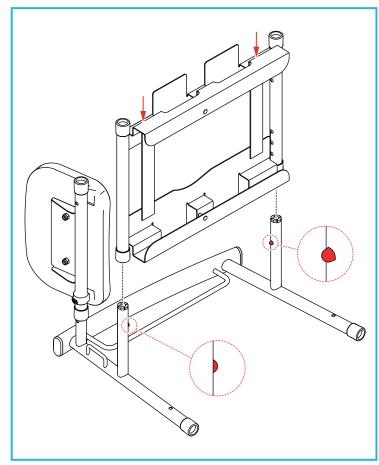
Slot the seat-frame assembly onto the LH sideframe assembly. Push and hold the button clips, then push down on the seat-frame assembly until the button clips click into the correct hole positions.
