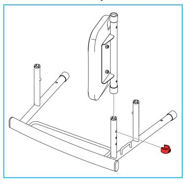
Slot the backrest assembly onto the side-frame assembly (LH) and secure with 1 x E-clip.
