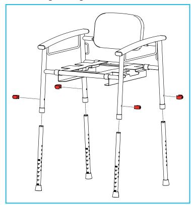
Insert the legs into the side frame assemblies and secure with 4 x E-clips.
