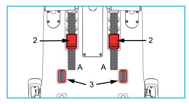
2. Feed the upper straps (A) down through the camlocks (2), then lock the camlocks closed.
