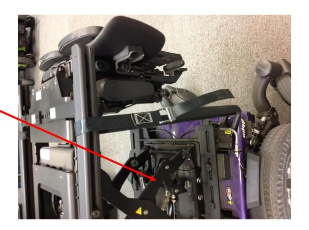
• Locate the front of the clevis pin on the tilt actuator.
