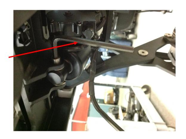
Slide tilt actuator back first over curved support bracket with motor facing right side of unit as seated in the chair.
