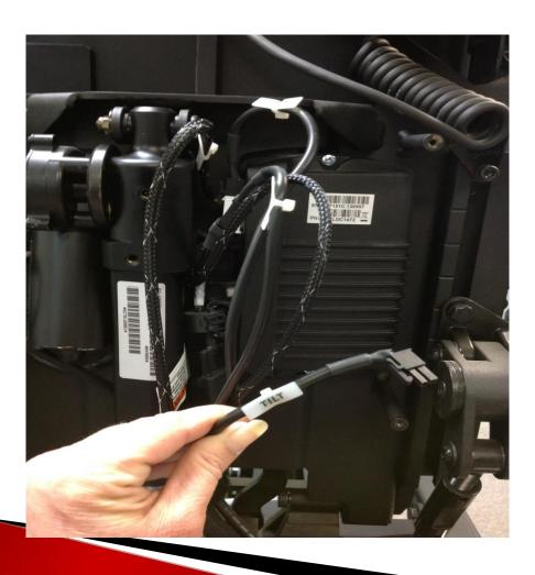
Unplug the tilt actuator from the seating module.
