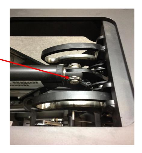
Remove the split ring and washer from the clevis pin using a snap ring pliers or two flat head screw drivers.
