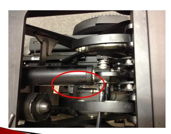
Tap the clevis pin out with a long screw driver & hammer.
