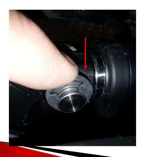
Install front clevis pin washer and spilt ring.
