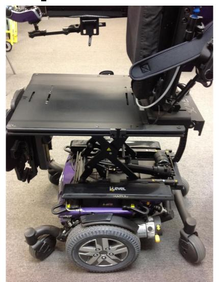
• Remove the (8) 4mm seat pan screws.
