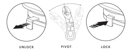
WARNING! Always monitor the user when the Pivot Plate is unlocked to rotate. The Pivot Plate should always be locked when driving the wheelchair or transporting it in a vehicle to prevent damage or injury that could result from striking doorways or other obstacles near the side of the chair.
