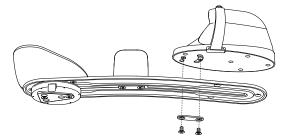
2. Mount the Hand Block to the Base Board using the Washer Plate and the included M6 screws (2).
